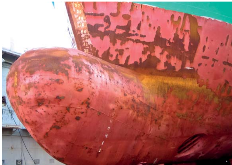
Ice going general cargo vessel. Left. The state of the hull after one season in the ice using a conventional coating, five years after the hull was originally coated but with the coating repaired on an annual basis. Center. Two years after Ecospeed was applied (no repair). Right. The state of the hull seven years after the Ecospeed application, with no repair in the meantime. The shipping company's manager of chartering points out, "There really is no other coating that could stand up to seven years of trading in ice and still remain intact and not in any need of repainting or anything beyond very minor touch-ups."
