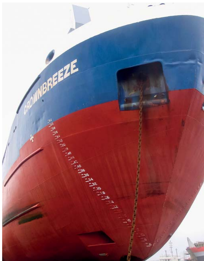
Ice going general cargo vessel. Left. The state of the hull after one season in the ice with a conventional ice coating, before Ecospeed was applied. Center. The same hull after 2 1/2 years of trading in ice in Baltic waters. Right. The condition of the hull 5 years after the initial application with no repair or repainting. Touch-ups of very minor mechanical damage to the coating in progress in drydock.
