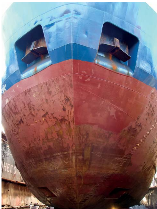
Ice going general cargo vessel. Left. The state of the hull after one season in the ice with a conventional ice coating, before Ecospeed was applied. Center. The same hull after 2 1/2 years of trading in ice in Baltic waters. Right. The condition of the hull 5 years after the initial application with no repair or repainting. Touch-ups of very minor mechanical damage to the coating in progress in drydock.
