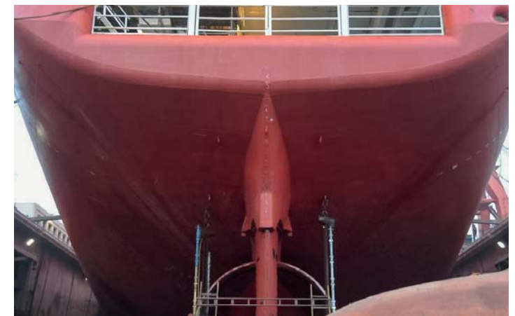
Right: Same ship after four seasons in heavy ice after Ecospeed was applied to the hull, with no repair or re-coating during those four years.
