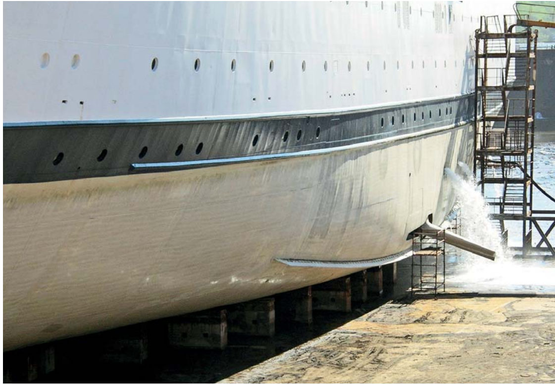
Hull of cruise ship after 5 years with Ecospeed coating with no replacement or major repair. This is the state of the hull when the ship came out of the water, without any cleaning or touch-up in drydock.
