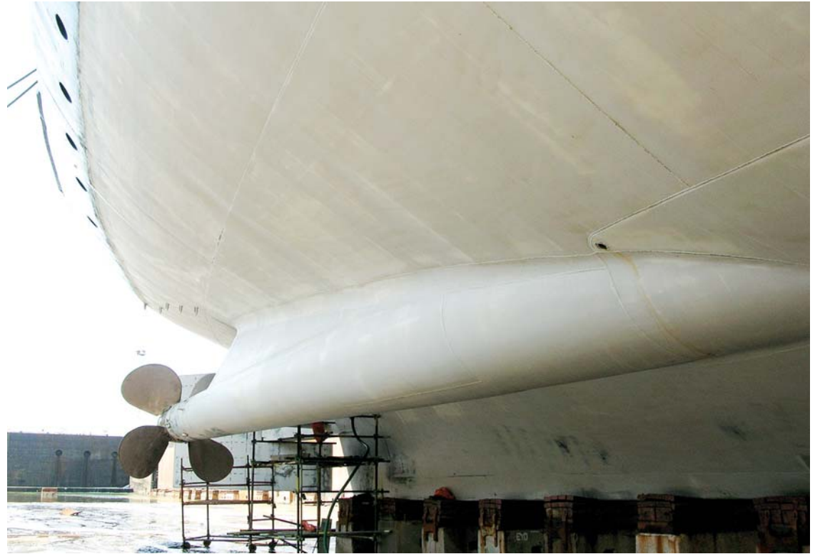
Hull of cruise ship after 5 years with Ecospeed coating with no replacement or major repair. This is the state of the hull when the ship came out of the water, without any cleaning or touch-up in drydock.
