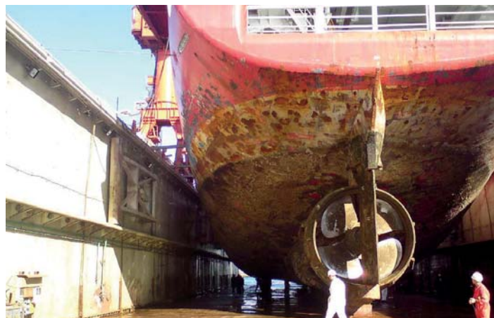
Left: RRS Ernest Shackleton, icebreaker and Antarctic supply ship, after a season in ice with conventional ice-going paint.
